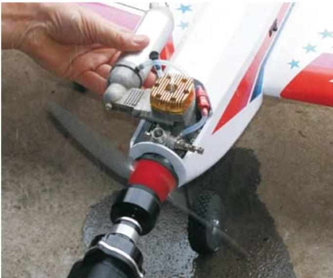
Remove the plug fill the cylinder with fuel and spin it over. Be careful, if it makes your eyes water that's bad.
