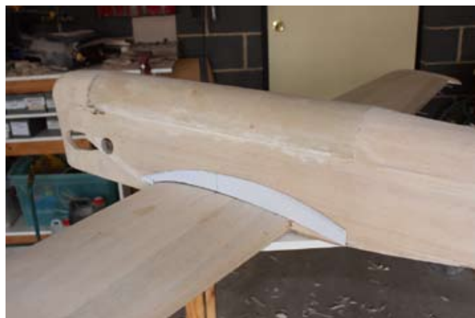
Marking out the wing section for wing fillet template
