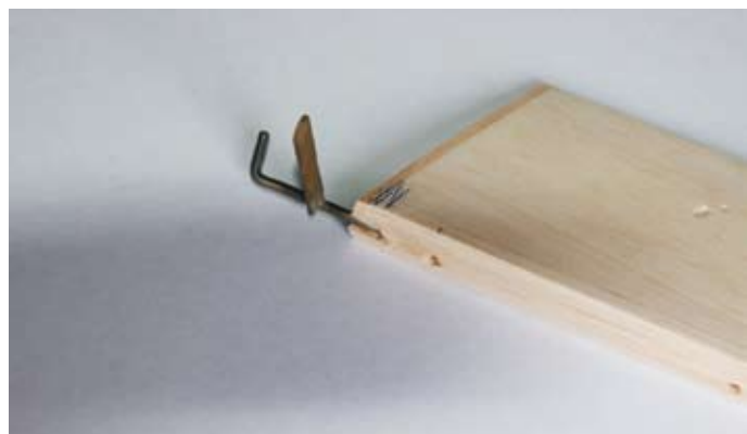
Internal elevator horn made from 5/32" (4mm) K&S spring steel wire. Plywood block yet to be added
