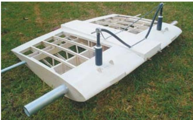
The undercarriage is a visual feature but bungee chord as on the full sized wasn't practical so we simulated it. The 8oz fuel tanks wouldn't fit in the nacelles and are built inside. The four nacelles took longer to make than any other part of the project.
