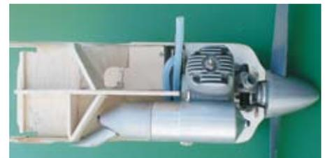
The simple and reliable OS 40 LA was the only engine considered. Only 30rpm difference between all four engines.
