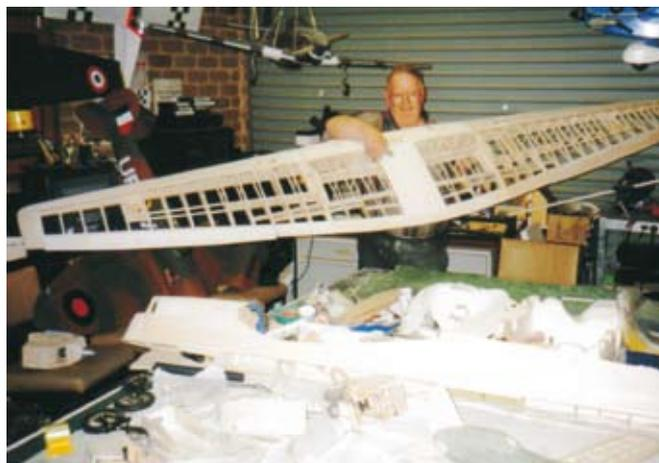
The wingspan is 3225mm which represents a 1.113.5 scale.
