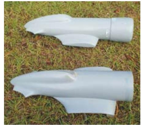
Very light fibreglass fuselages for the fourth attempt at reducing weight in Pokilov fighters.
