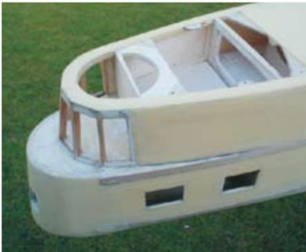
The slab sided fuselage was simple enough and although the strange glazing took a bit of working out everything else in cockpit was fun modelling.
