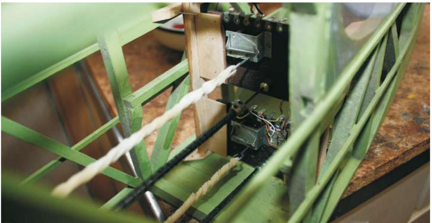
Rubber bands are in effect pushrods, driven by an "Escapament" Left twist one way - right the other. Ditto for elevator. Fly too long and use too many control inputs, the rubber band runs out of turns. Inherently stable free flight design took over and the model continued on flying. Wherever it wanted!
