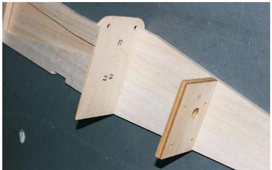
Fuselage sides milled for the bulkheads
