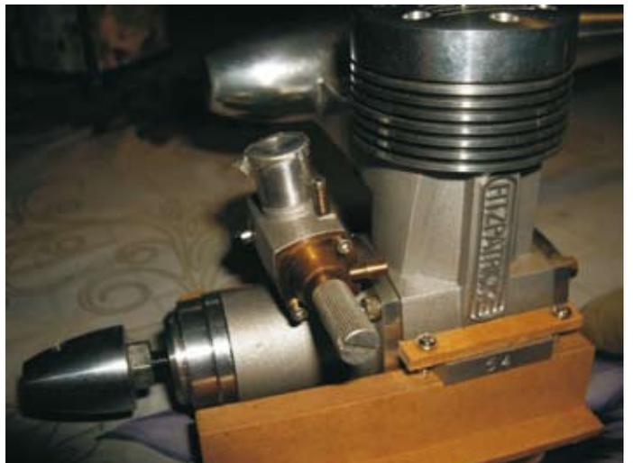
Fitzpatrick 61 NVA uses 2 O rings side by side to seal & stop NV from moving when running
