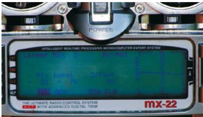
Rudder to aileron mix, 5% left and 7% right.
