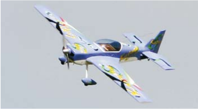
In a side slip keep the rudder constant and steer it in with elevator and aileron. The low wing goes into wind.
