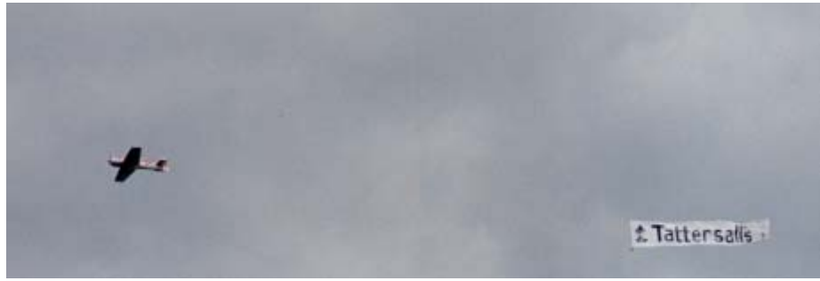
Like towing a caravan at Winton V8 Supercars. Up elevator trim was free mixed with the release. When the tow line snagged in the elevator counterweight we decided a dedicated banner tow plane was needed.
