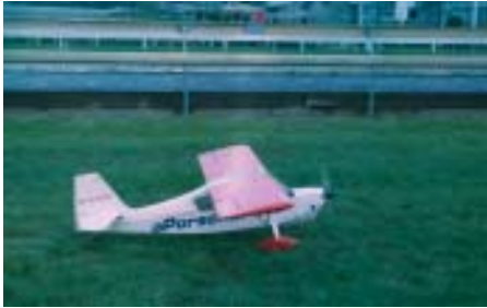
Swapping the 23cc mil for a 74cc twin cylinder gave it plenty of power for banner towing.
