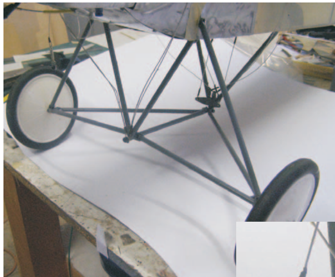
The upper pylon that supports the wing warping cable pulley and the landing wires that attach to the front spar. The aluminium skin is lithoplate that is burnished with a small wire brush in the Proxxon drill.
