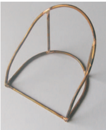
The pilot's seat frame is from 1/8 brass tubing silver soldered up. To be clad in litho plate and then leather.
