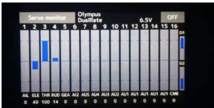
Channel 2 indicates holding full up elevator with Dual Rate selected
