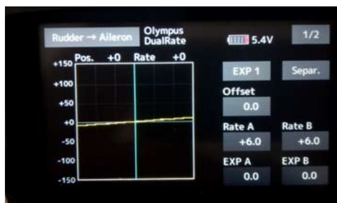
Rate A and B are left and right aileron
