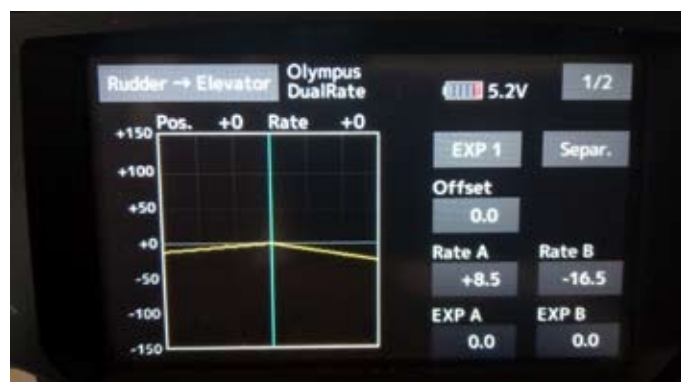
Rate A and B are each elevator input for left and right rudder
