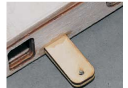
Wicking in thin cyano is the easiest way to prevent this coming loose
