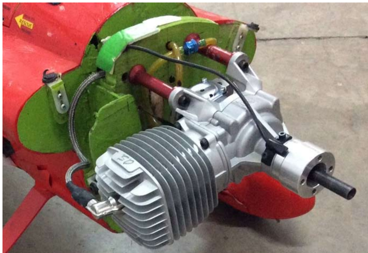
Fire-wall replaced with two pieces of 6.5mm aircraft or marine grade plywood with 1.5 mm ply doubler each side of the engine box
