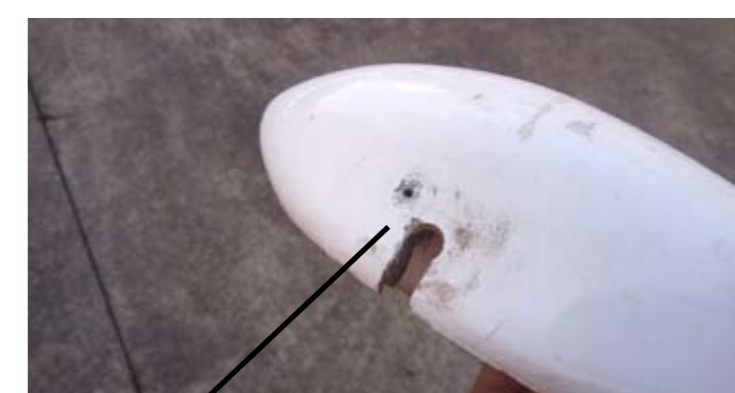
Bolt drilled through undercart leg acts as anti rotation pin
