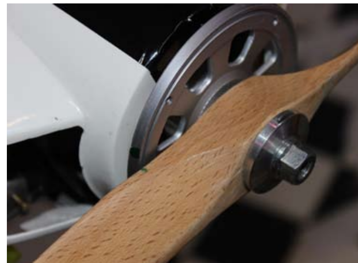
Green mark on back plate makes alignment easier
