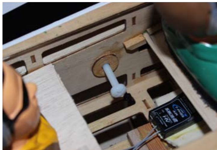
Keep an eye on the wing bolt torque
